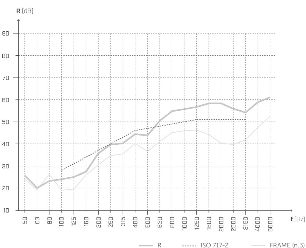
$$R_w(C, C_{tr}) = \text{47} \text{ (-2;-8) dB}$$
