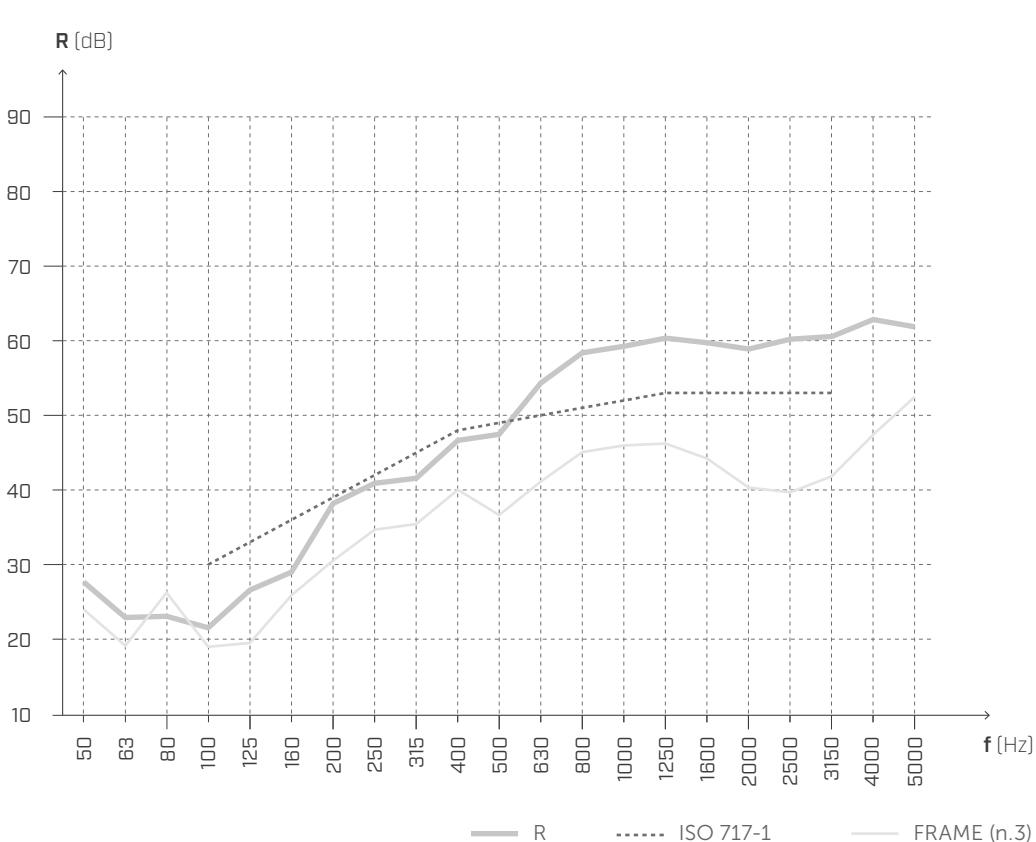
$$R_w(C, C_{tr}) = \text{49} \text{ (-3;-10) dB}$$
