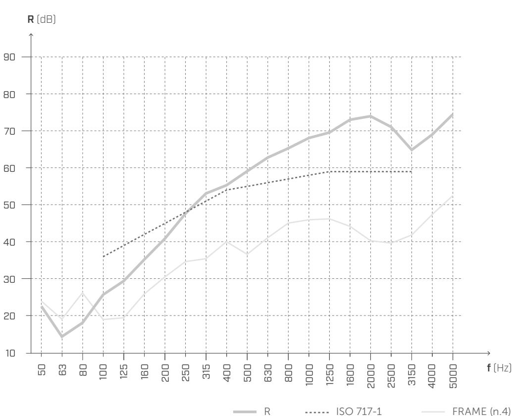
$$R_w(C, C_{tr}) = \text{55} \text{ (-5;-12) dB}$$
