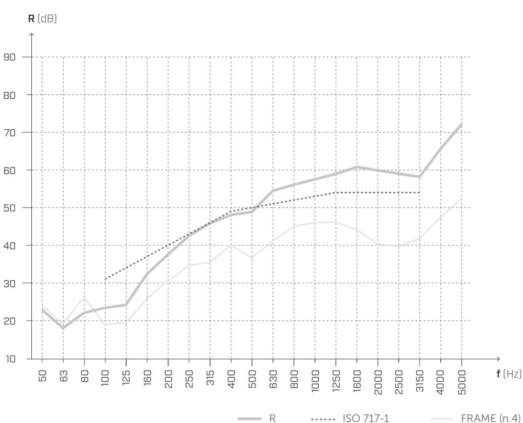
$$R_w(C, C_{tr}) = \text{50} \text{ (-4;-10) dB}$$
